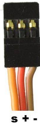
Figure 7: Servo pinout: s to D9 on the board or PORTB1, + to VCC, - to GND
